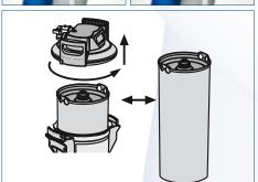
Thanks to the innovative 'Quick Lock' principle, the pressure vessel can be opened very easily. Thanks to the water shut-off valve in our standard hose sets, the filter cartridge is changed in a trice – without tools and with little effort directly at the filter: you remove the pressure vessel lid, take out the used cartridge, insert the new cartridge and put the lid back on: done!
